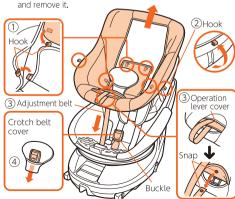
\* Remove the canopy from the headrest before removing the seat cover. (Refer to "Removing the canopy" on page 25.)
