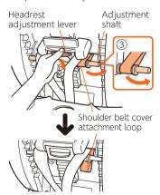
4 Unfasten the snaps of the shoulder belt cover and pull the cover forward to remove it
